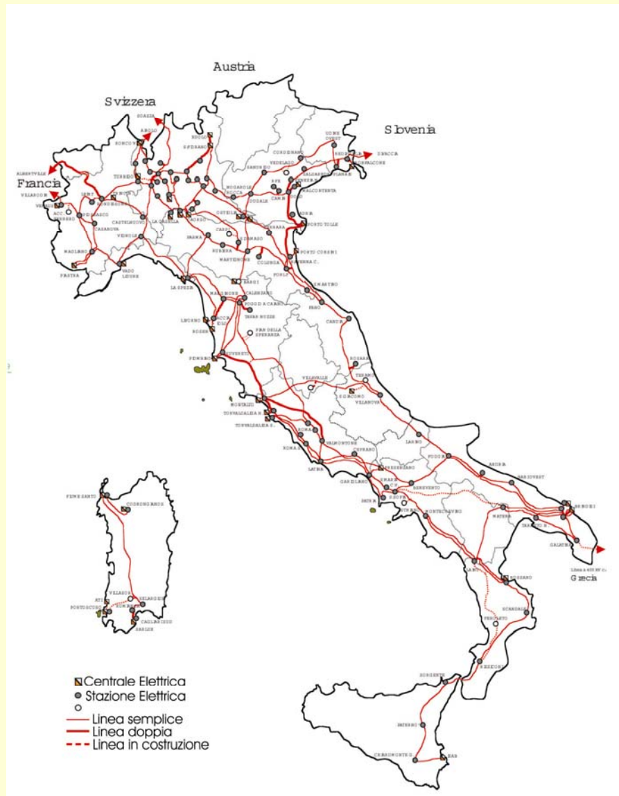
The Italian high voltage electric network (380.000 V)
